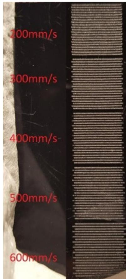
To compensate for this, measure the distance between the ends of the lines at each speed, and enter the speed and distance values into the scanning offset adjustment table. LightBurn will use this information to compute the correct adjustments for other speeds as well. A minimum of two measurements are needed for it to work.
