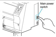
The firmware version is displayed when the power is turned on.
