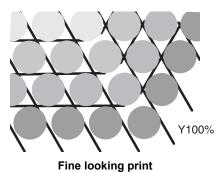
In the blue area (100% magenta + 100% cyan), however, speckled patterns and banding occur. This banding is a result of beading. If heater temperatures are low or the ink capacity (ink limit) of the media is low, the first dot does not solidify before the second dot lands on the media. As a result, dots bond to each other and unevenness or banding occurs.
