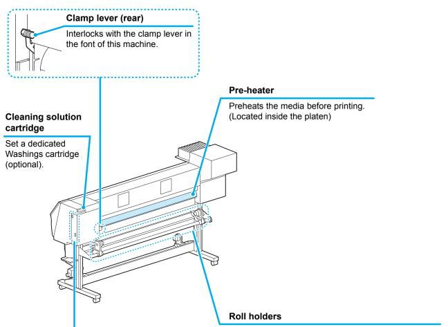
Hold a media by inserting it into the right and left ends of the core of the roll media. Roll holders are available for the 2 inches and 3 inches core of the roll media.
