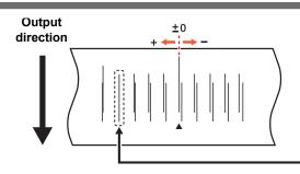
The dots at the fourth position counted from the zero position in the positive direction form a straight line. In this case, the dot position correction value is 4.0.
